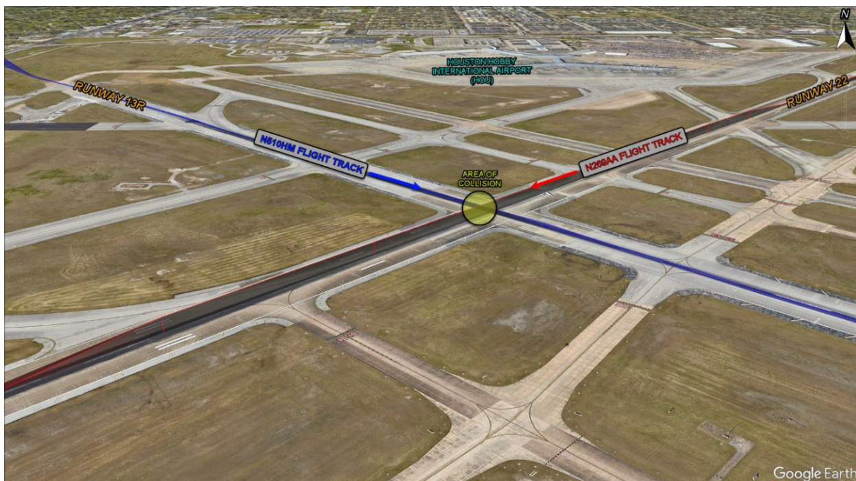
Figure 1. View of both airplanes flight tracks with the area the ground collision occurred highlighted in yellow. The blue line represents N510HM, and the red line represents N269AA.
