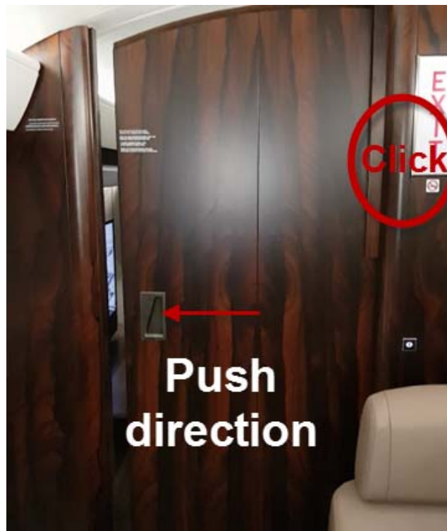
Figure 5 – Restoring Normal Operation of Sliding Door
